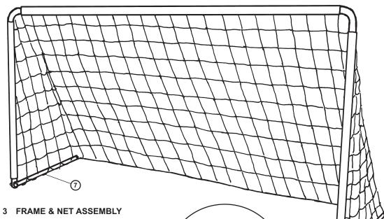
Being careful to select the appropriately numbered tubes (tube 7), thread tube 7 through the net and attach to the base of tube 4 using a long bolt as illustrated.
