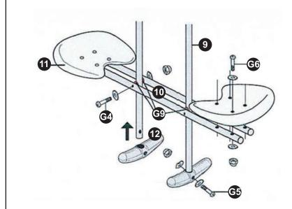
• Assemble seats (11) and attach to seat tubes (10) before tightening bolts (G4)
