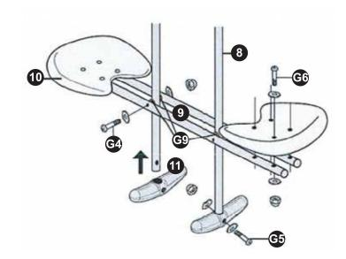
• Assemble seats (10) and attach to seat tubes (9) before tightening bolts (G4)
